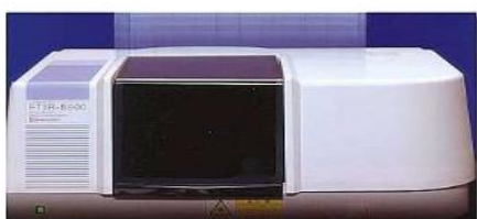
Figure 5 Fourier Transform Infrared Spectrometer (FTIR – 8400 Shimadzu)
